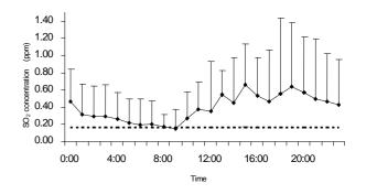
**Figure 2.** Variation of the hourly concentration of  $SO_2$  in greenhouse air (mean  $\pm$  S.D.) during eight measured periods, related to the hourly threshold limit value (dotted line).
