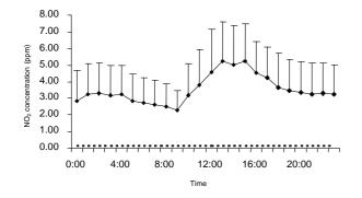
**Figure 1.** Variation of the hourly concentration of  $NO_2$  in greenhouse air (mean  $\pm$  S.D.) during nine measured periods, related to the hourly threshold limit value (dotted line).
